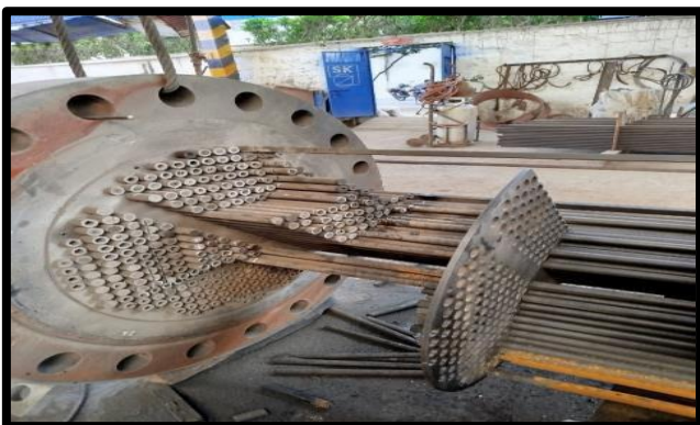
Bundle Tubes cutting/ New tubes Cold Bending
