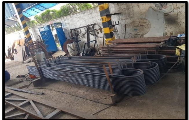
Bundle Tubes cutting/ New tubes Cold Bending
